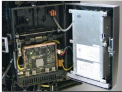
Control unit can be opened while the tile is operational
