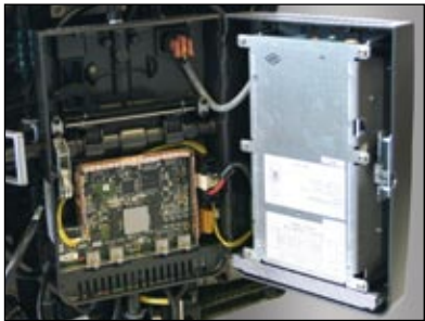
Control unit can be opened while the tile is operational. The same control unit is used on both NX-6 and NX-4.
